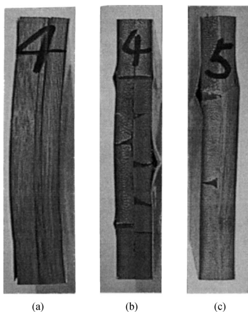
Figure 9 Photographs of failed PAB compressive test specimens: (a) L, (b) T and (c) C orientations.
